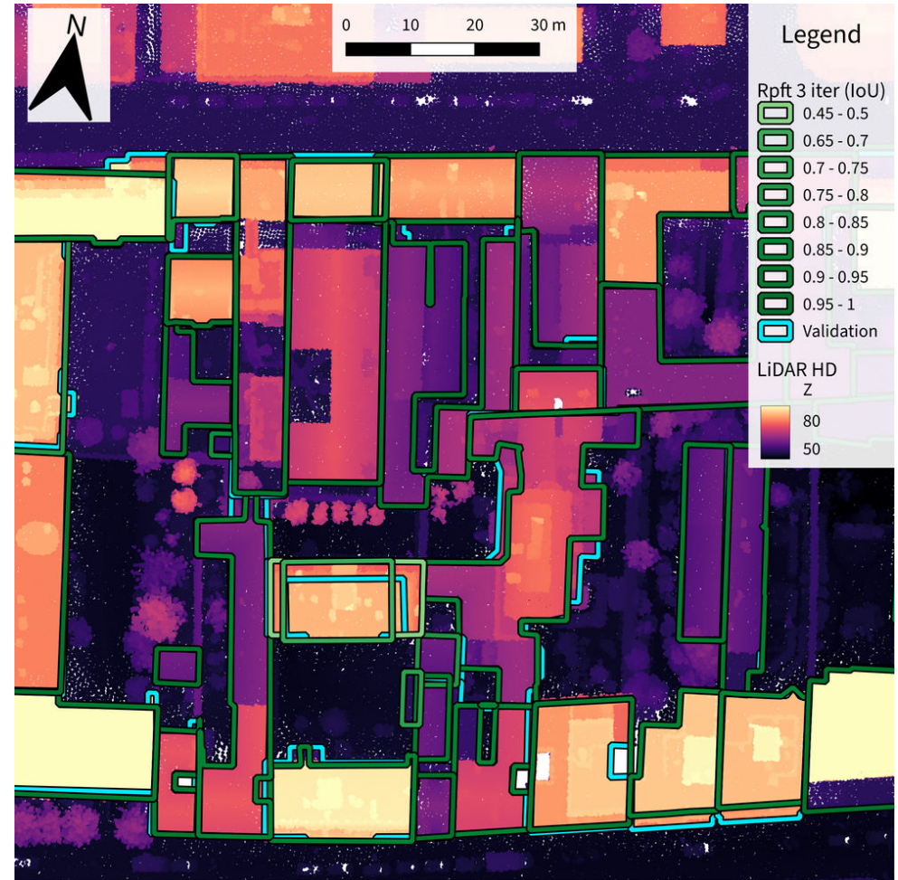
Figure 24: Roofprints after 3 iterations.
