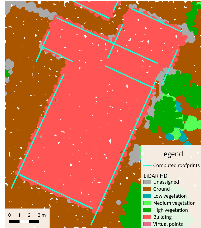
Figure 13: Comparison of BD TOPO outlines and computed roofprints.
