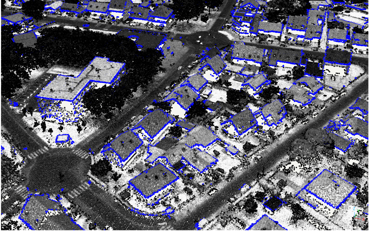
Figure 7: Edge points in blue and LiDAR HD data in gray scale from low (black) to high (white) intensity.
