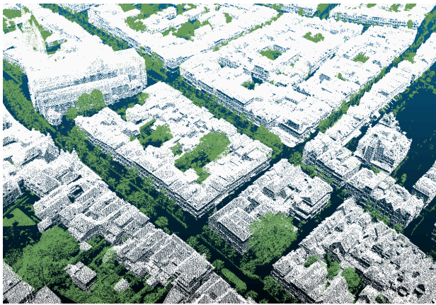
(c) First example: the point cloud from AHN 4 filtered to keep only "Not classified" (green) and "Building" (white).
